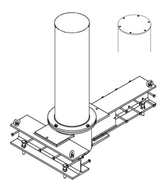
**Design:** Removable blocking bollard(s) with base supports for shallow mount
